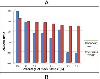
**Figure 3.** The sensitivity of spectrophotometry instrumentation. A high quality HeLa RNA sample was serial diluted, and measured via nanospectrophotometry (NanoVue, GE Healthcare) or via cuvette-based spectrophotometry (Ultraspec 2100 Pro, GE Healthcare). A) The sensitivity of both spectrophotometers based on the percentage of the stock HeLa RNA sample, determined using the A260:A230 reading. B) The sensitivity of both instruments based on the A260:A280 ratio.
