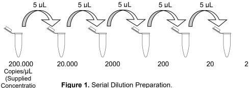
Figure 1. Serial Dilution Preparation.
